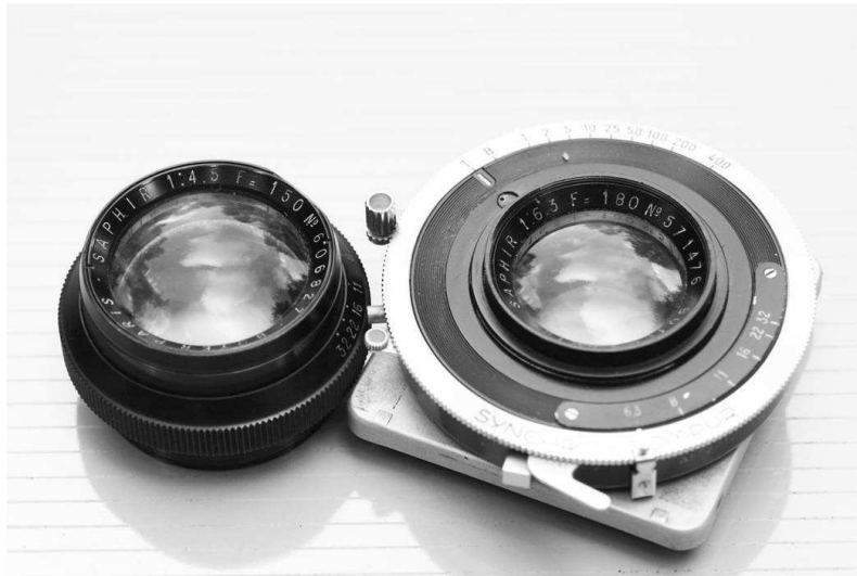
Figure 7: Tessar type Saphirs, 4 elements, f/4.5 150 mm and f/6.3 180 mm ( photo C. Barringer )
