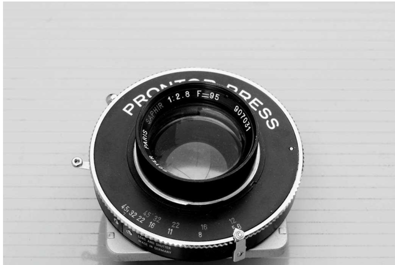
Figure 6: Saphir lens, 6 elements double Gauss, F/2.8 95 mm ( photo C. Barringer )
