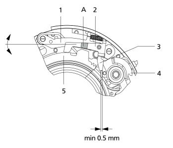
1 Bridge 2 Locking lever 3 Nose of locking lever 4 Drive 5 Cocking ring
