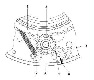
1 Borehole 2 Intermediate cocking gear 3 Cocking shaft 4 Mark 5 Index 6 Spring for intermediate cocking gear 7 Spring suspension rivet
