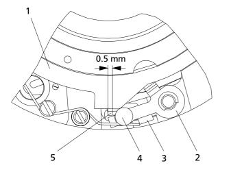
1 Cocking ring 2 Control lever 3 Fin 4 Rivet 5 Control latch
