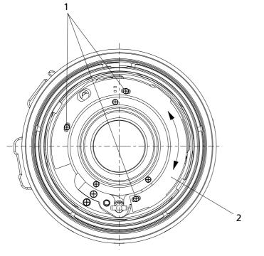
1 Screws 2 Printed circuit board
