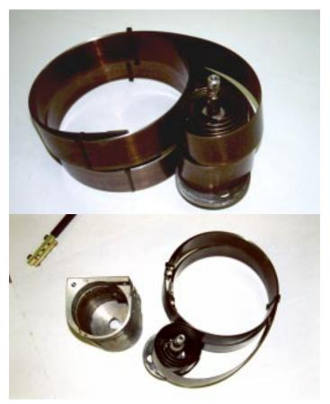
The front plate on the spring housing is 4mm thick plate aluminum. If the spring is allowed to uncoil uncontrolled it will knock off this plate, ripping ALL SIX 4mm screws from their sockets.
