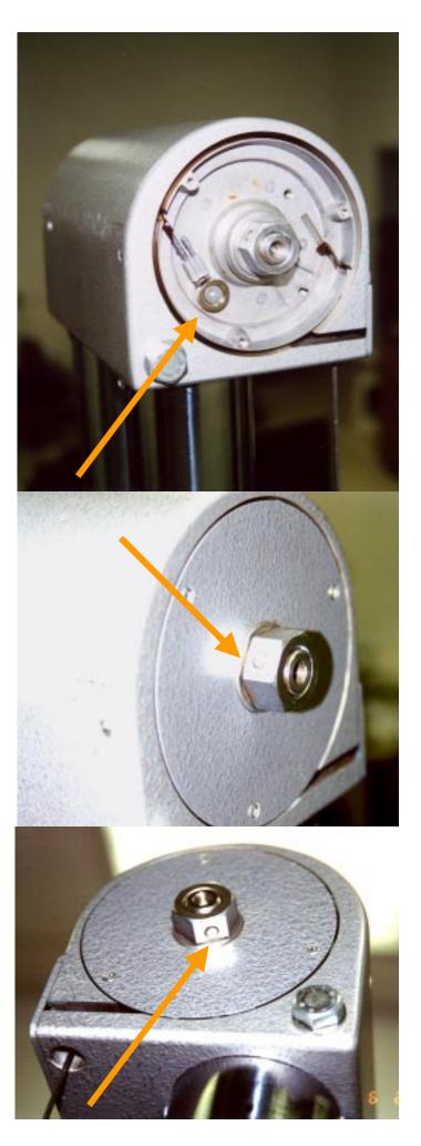
When the wire disk in the right side has been removed and the wire hanging loose it is possible to bring the tension tool back to a position where it is parallel with the column and then remove the "C" bracket.
