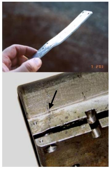
On this picture you will see the effect of a spring accident. The force of the spring knocked the  $\frac{1}{2}$  - 1" thick aluminum housing almost  $\frac{1}{2}$  inch out of shape.
