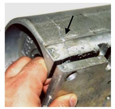
If you look careful at the image below you can see that the entire 10 pound aluminum housing has been knocked out of shape by more than 1/4". The aluminum housing is 1/2" thick at its thinnest place. The force released by an uncontrolled spring is several thousand pounds
