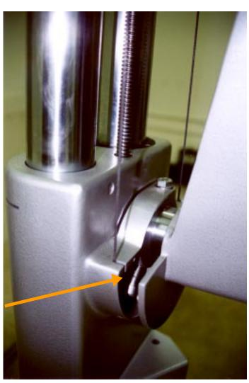
In order to remove the camera on an L184 it is only necessary to remove one screw. When this screw is removed the camera will slide off the support arm. Here it is also helpful to be two persons, one person to hold on to the chassis and one to pull the camera off. The camera is quite heavy, be careful not to drop it
